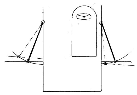
If the T.A.s are tapered, the resultant skew can be used to counteract the steer resulting from Figure 1. The effect is greater on the top arms as they are further from the Roll Centre.
